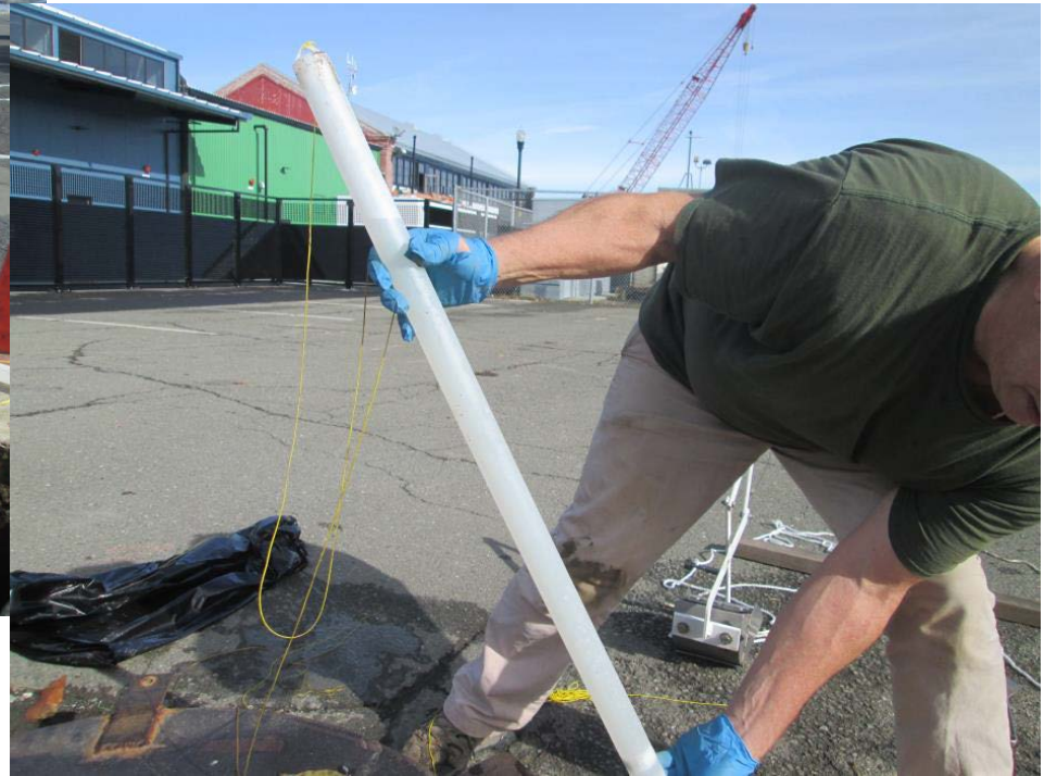
Water Sample Collection with Bailer
