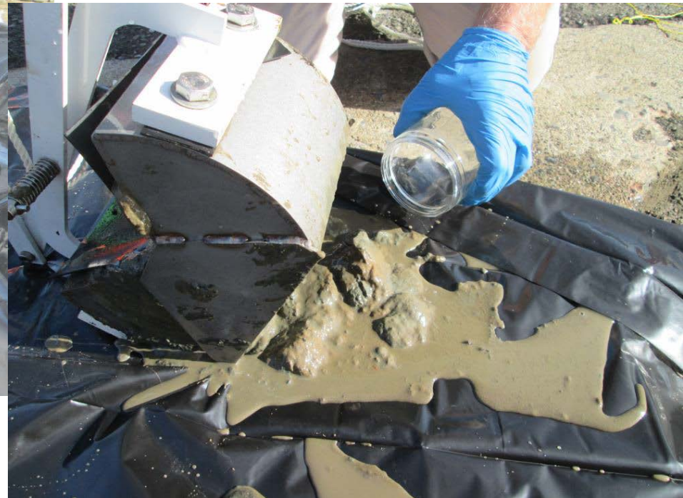
Sediment Collected from Southern CWL-IA Pipeline
