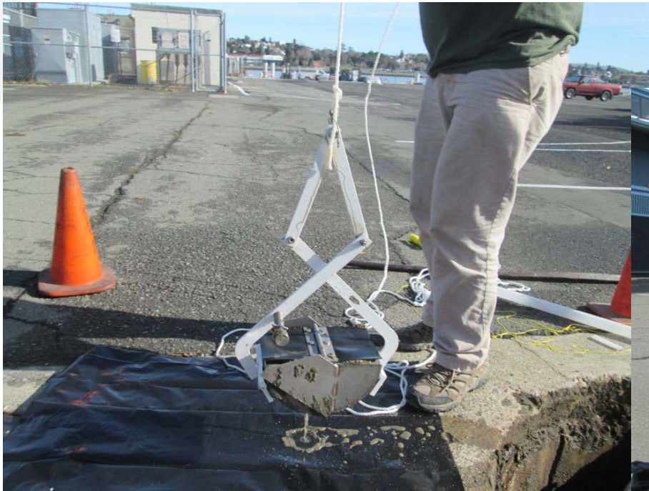
Sediment Sample Collection with Clam-Shell Sampler
